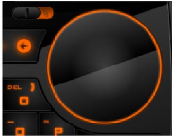
In touch-pad mode, the ClickPad functions like a touch pad. On-screen cursor navigation is done by moving a finger across the ClickPad, which is perfect for Web surfing or other traditional computer operations. Note the orange backlit ring around the ClickPad.
